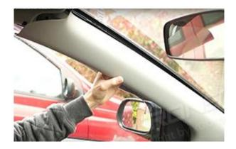
Scratch away some paint from the A Pillar to attach the copper grounding lug. (Please tear out the sticker from the grounding lug surface and ensure the grounding lug has good conduction with the car's ground).
