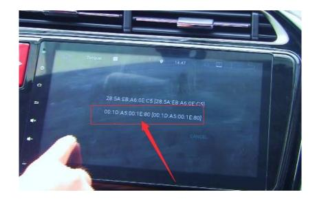
7. Return to the OBD mode on the head unit, it might take 30 seconds for OBDII connecting successfully.
